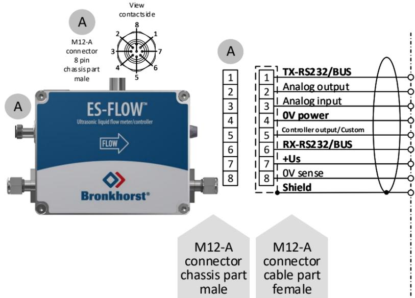
⚠ When connecting the system to other devices, be sure that the integrity of the shielding is not affected. Do not use unshielded wire terminals.
