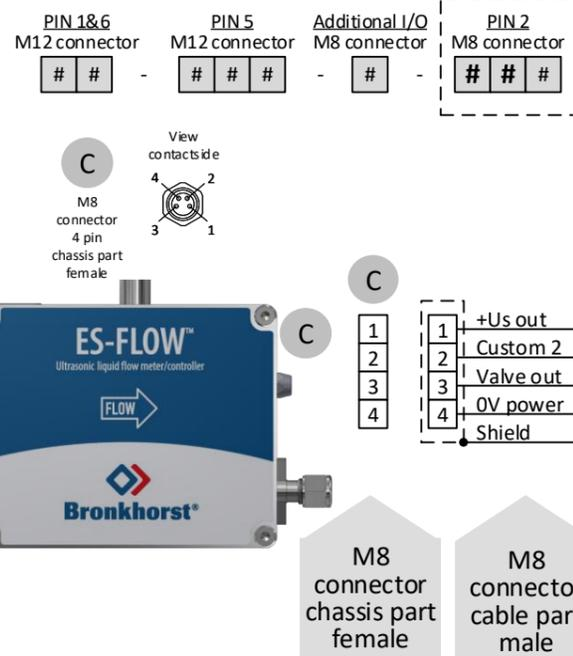
⚠ When connecting the system to other devices, be sure that the integrity of the shielding is not affected. Do not use unshielded wire terminals.
