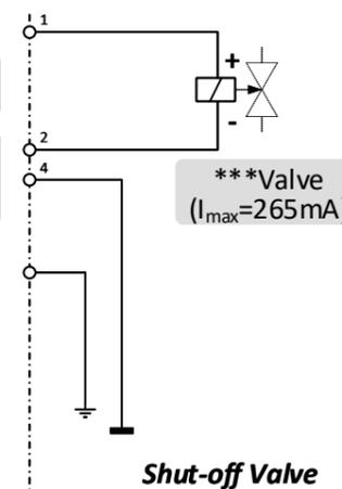
Note: \*\*\* For 15Vdc supply the minimal Load is 60  $\Omega$ , for 24Vdc supply the minimal load is 90  $\Omega$
