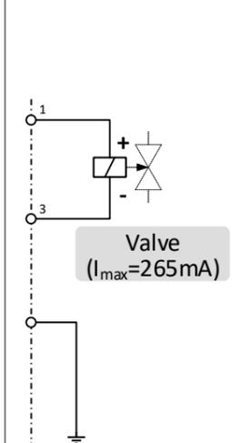
Internal setup digital output
