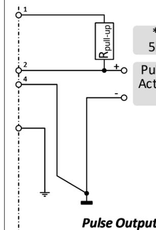
Note: \* Use  $R_{pull-up}$  (between 5k $\Omega$  and 10 k $\Omega$ ) to create 15-24Vdc at PIN 5
