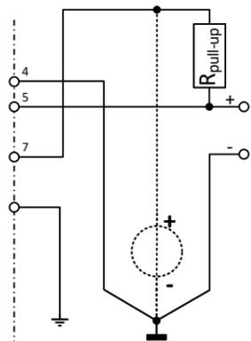
\*  $R_{pull-up} = 5k\Omega - 10k\Omega$
